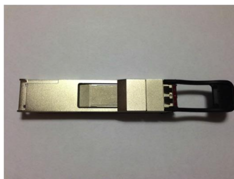
Figure 2. Cisco QSA Module with SFP or SFP+ Plugged In
