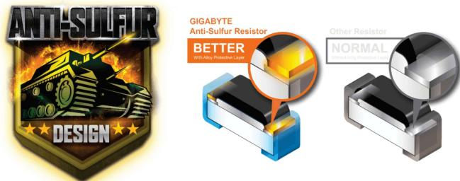
Sulfur compounds in the air can penetrate tiny onboard resistors creating chemical change and causing these resistors to open or short. If either of these occurs the motherboard will fail to function. By equipping resistors with an Anti-Sulfur Design GIGABYTE gives Ultra Durable Motherboards a whole new meaning.
