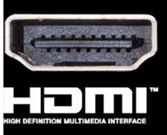
HDMI 2.1, which is backwards compatible with HDMI 2.0/ 1.4 and offering 48 Gb/s of bandwidth – twice times more than previous generation. This unlocks the potential for users to transfer multiple video streams, as well as a native cinematic 21:9 ratio (which most movies are shot in), Full HDR and HDCP 2.3 support, to offer the best visual experience for viewers.
